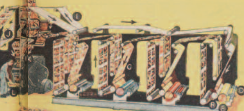
(18) ROTARY PHOTOGRAVURE PRINTING MACHINE. (A) Paper reel; (B) First colour printing, one side only; (C) Paper passes to the other end for colour printing on reverse side; (D) Ink scraper or doctor blade; (E) Printing cylinder and ink reservoir; (F) Impression cylinder holding paper against printing cylinder; (G) Second colour printing on reverse side; (H) Web is now split by a cutter into page width and parts company on its way to the folder; (I) In the meantime, the black and white section is being printed on one side at the back of this machine and passes right over to the left to be printed on the other; (J) The black printing returns and is split; (K) The four split webs come together and are cut and folded into 8 sheets; (L) Delivery of copies.
